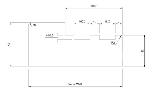
Do Not Scale. Description: Purchasing Profile Timber System 2 - 44\_32 Profile - FD60 - 55mm Door - Acoustic - Non Q2F If In Doubt Ask!
